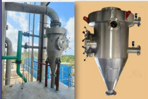
MIST TYPE WATER JET VACUUM CONDENSER (MTWJVC)
